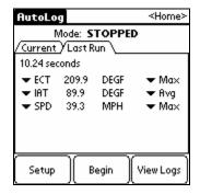
In this example, the engine coolant temperature reached a maximum of 209.9 degrees F, the average intake air temperature was 89.9 degrees F, and the maximum vehicle speed was 39.3 MPH. Click on a parameter name or the word "Max" to change the display. Note that only the parameters that were selected to log will be included here. For instance, if KR (knock retard) was not included in parameter list 1, then you can't view the Min, Max or Avg value of KR during this run.
